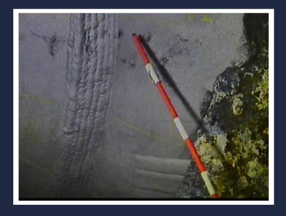
Historically inspection pointers for divers have been cobbled together using welding wire and electrical tape. Whilst this method has been adopted the pointers vary in shape, colour. Size of graduation differs from one pointer to the next. Often with damaged pointers starting to unravel.
